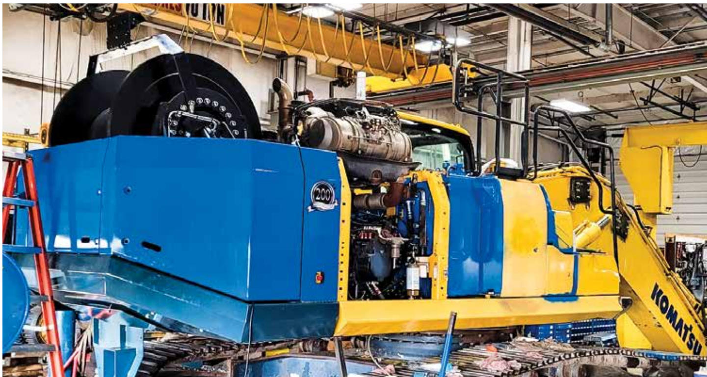
After removing the counterweight and thoroughly inspecting the machines, Modern Machinery service technicians mounted the Falcon Winch Assist on the back of the excavator, which gave it approximately the same operating weight as a traditional excavator. The Falcon Winch Assist houses about 1,640 feet of 1 1/8-inch swaged rope with nearly 80 tons of breaking strength.
