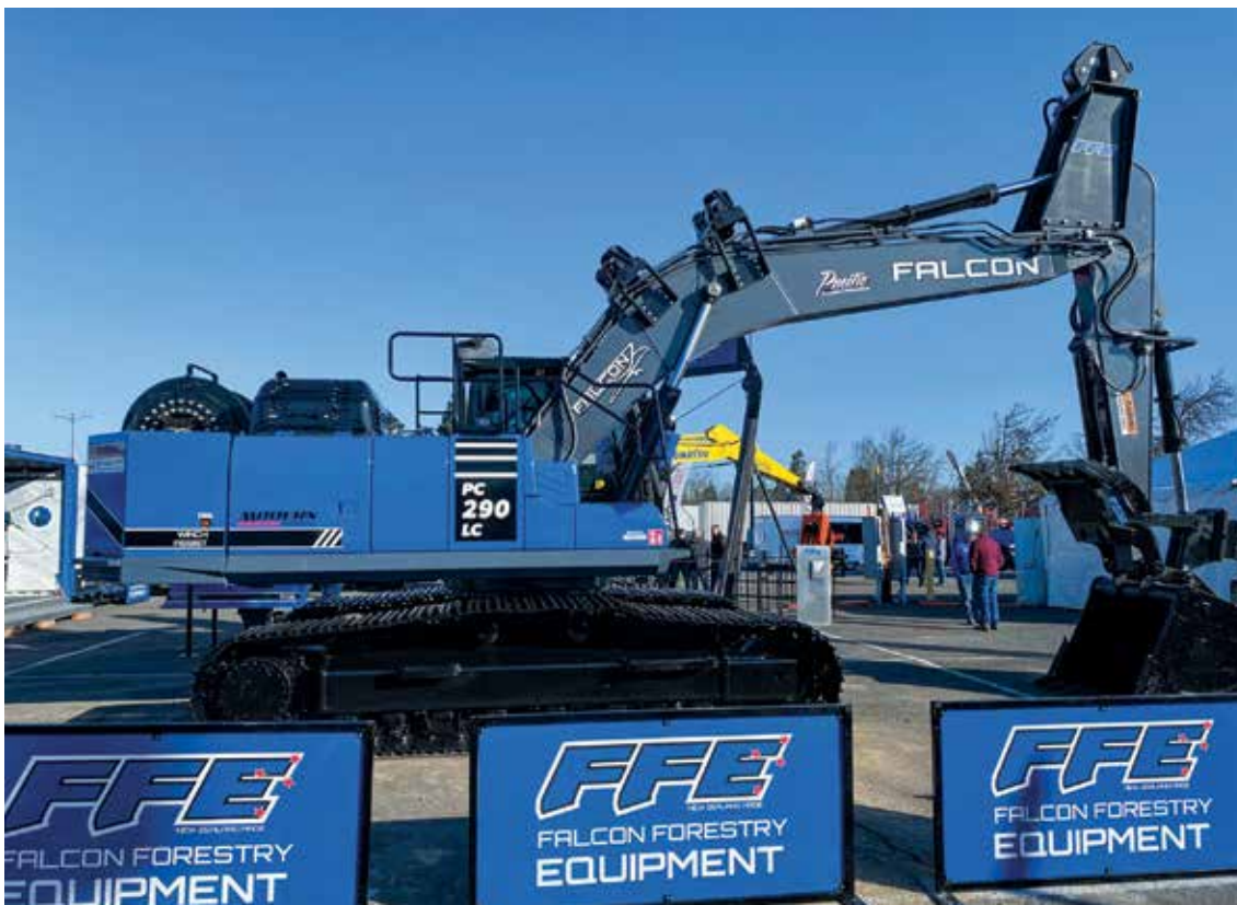
Modern Machinery's booth featured the Falcon Forestry Equipment steep-slope, winch-assist machine on a Komatsu PC290LC-11. The Falcon set up is designed for safer operation where it would be too dangerous to work without cable assist.
