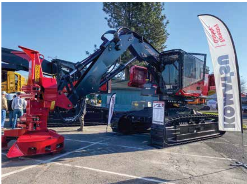
The TimberPro TL755 "West Coast Special" was another highlight of Modern Machinery's display. It was equipped with a Quadco 27B 360-degree saw head.
