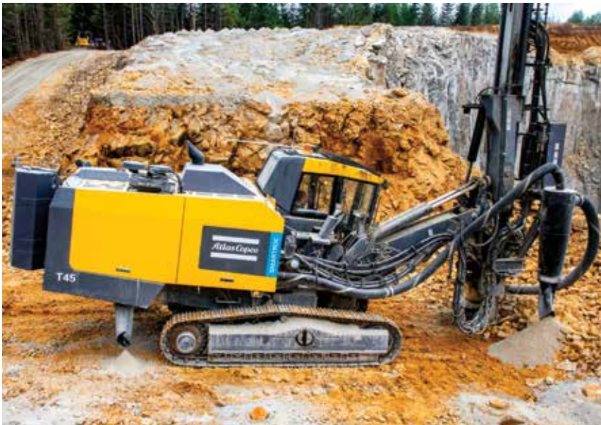
J.L. Storedahl & Sons recently acquired this Atlas Copco (Epiroc) SmartROC T45-10 to drill blasting holes.
