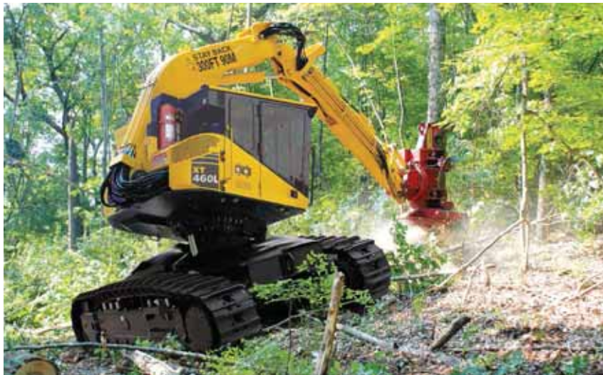
Four sizes of forestry tracked harvesters and tracked feller bunchers are produced at Komatsu's CMO, among them are new Dash-3 models, including the XT460.
