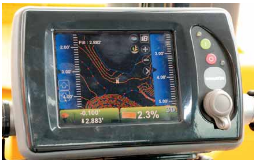
The integrated intelligent Machine Control system features stroke-sensing cylinders and a cab-top antenna that eliminate the traditional mast(s) and cables associated with 3D machine control. Operators can also select modes to match material conditions.
