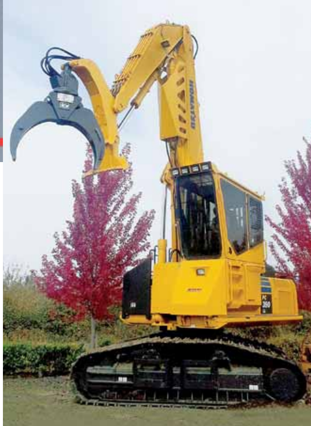
Don Miller is the primary operator of Weist Logging's new Komatsu PC390 log loader. "It's got a shorter track so it's easy to maneuver, but still very stable, which is important since we're often on steep ground," said Miller.
