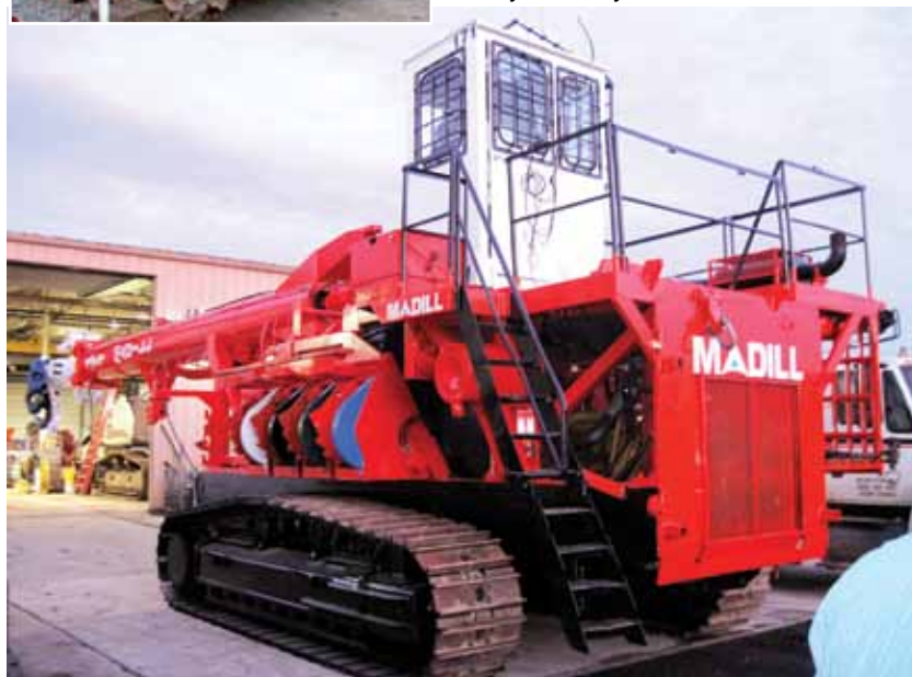
This Madill 171 yarder (left) was severely damaged after going over a cliff. Modern Machinery rebuilt the unit to a “like-new” condition (below) that includes numerous upgrades from the original yarder. Among the upgrades is a new, excavator-type hydraulic undercarriage to replace the old, tank-style track system.
