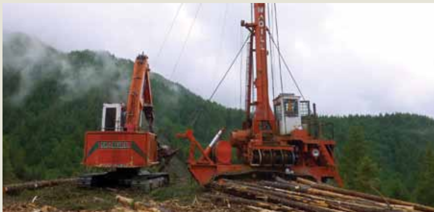
Dilley & Soloman's rebuilt Madill 171 yarder (right) works at a job near Forks, Wash. "With the new undercarriage and other upgrades, it's a better machine than when it was new," said Lyn Soloman. "We're very pleased with it."
