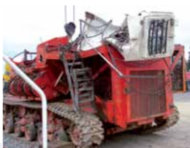
This Madill 171 yarder (left) was severely damaged after going over a cliff. Modern Machinery rebuilt the unit to a “like-new” condition (below) that includes numerous upgrades from the original yarder. Among the upgrades is a new, excavator-type hydraulic undercarriage to replace the old, tank-style track system.
