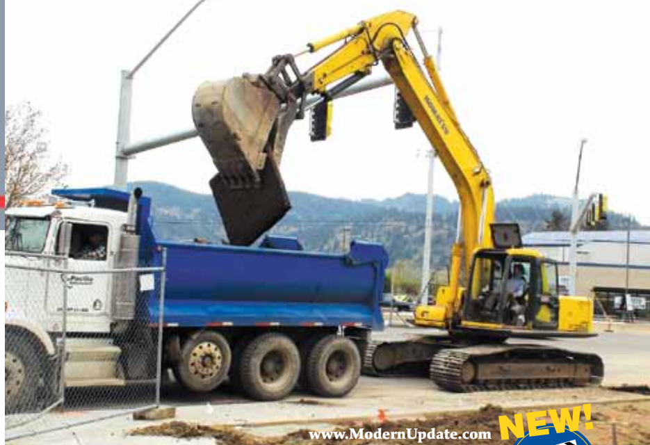
Pacific Excavation relies on Komatsu excavators in both its site-work and heavy-civil divisions. Here, an operator uses a PC220LC to load a truck with broken concrete from a street job.
