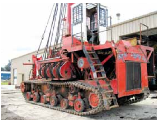
Modern Machinery refurbished this older Madill model 171 yarder (left), converting the old drive system to a modern crawler undercarriage. The refurbished unit (below) offers better mobility, higher productivity and lower cost of operation.
