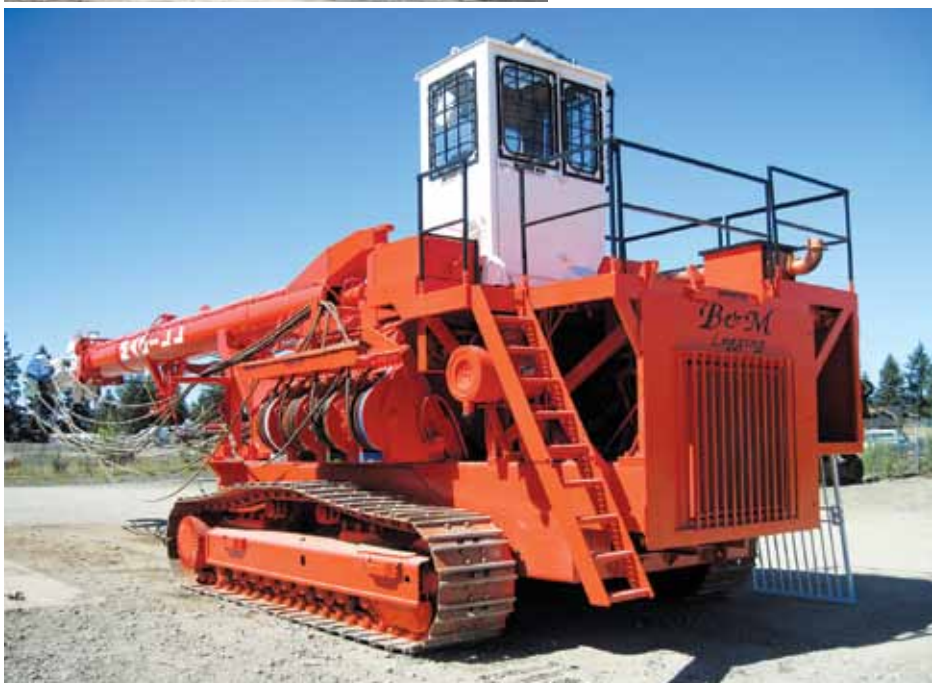
Modern Machinery refurbished this older Madill model 171 yarder (left), converting the old drive system to a modern crawler undercarriage. The refurbished unit (below) offers better mobility, higher productivity and lower cost of operation.
