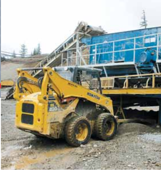
This ECP operator uses a Komatsu SK820 skid steer loader to clean up under the company's mobile crusher.
