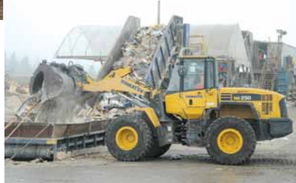
(Above) This United Recycling operator uses a Komatsu PC300LC-7 to feed wood waste into a grinder. (Left) United has three Komatsu WA250 wheel loaders to handle construction and demolition debris.
