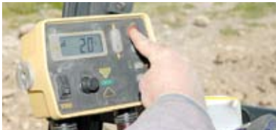
Mounted on a Komatsu PC50, the SGS 2000 uses a TOPCON control system to achieve rough grade that's within one-fourth inch of finish grade. "We've found the Komatsu PC50 to be the ideal carrier for the SGS 2000 because of its hydraulic power, strength and overall reliability," said Co-owner Steve Schmidt.
