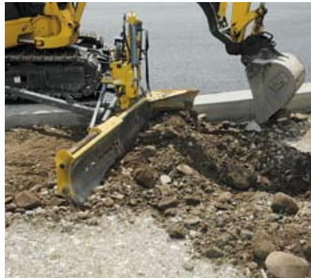
Mounted on a Komatsu PC50, the SGS 2000 uses a TOPCON control system to achieve rough grade that's within one-fourth inch of finish grade. "We've found the Komatsu PC50 to be the ideal carrier for the SGS 2000 because of its hydraulic power, strength and overall reliability," said Co-owner Steve Schmidt.
