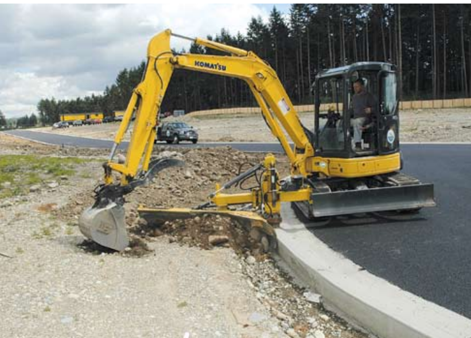
Mounted on a Komatsu PC50, the SGS 2000 uses a TOPCON control system to achieve rough grade that's within one-fourth inch of finish grade. "We've found the Komatsu PC50 to be the ideal carrier for the SGS 2000 because of its hydraulic power, strength and overall reliability," said Co-owner Steve Schmidt.
