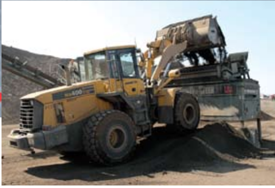
Foreman Dave Cox uses a Komatsu WA400 wheel loader to feed a crusher at High Banks Sand & Gravel, one of five pits Johnny Cat operates in southern Oregon.
