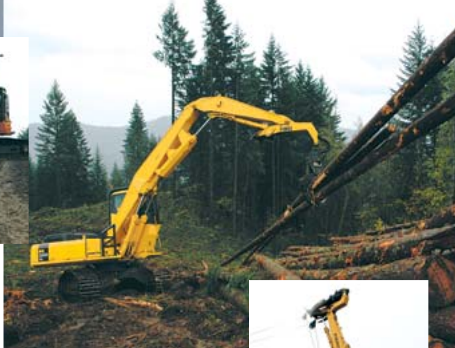
Ramco uses its Komatsu PC300LL-7 at the Ariel job as a shovel logger, getting trees from the woods to the landing for processing.
