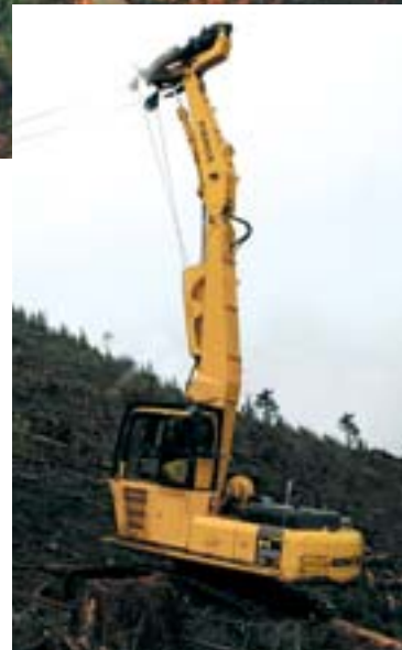
Ramco has two Komatsu PC300LL-7 log loaders, including this one equipped with winches and drums for use as a downhill yarder to clean up on steep, corner slopes, like this job near Mount St. Helens.
