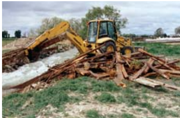
J & C Custom has a Komatsu WB140 backhoe loader for miscellaneous work, including removing debris from a stream.
