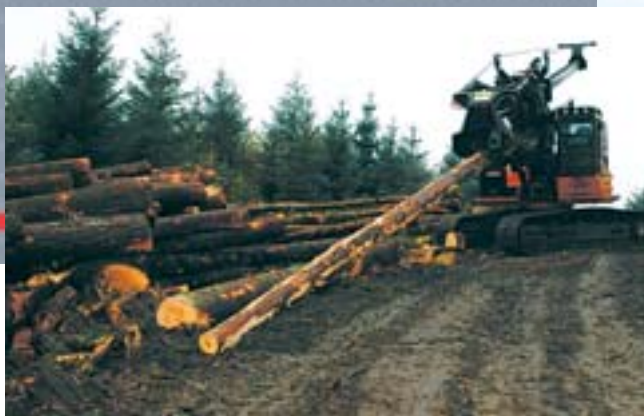
A pioneer in mechanical tree harvesting, Ramco does both cut-to-length and clear-cut work. Here, a Ramco operator uses a Pierce-Pacific stroke delimeter at a job for a private landowner in Ariel, Wash.
