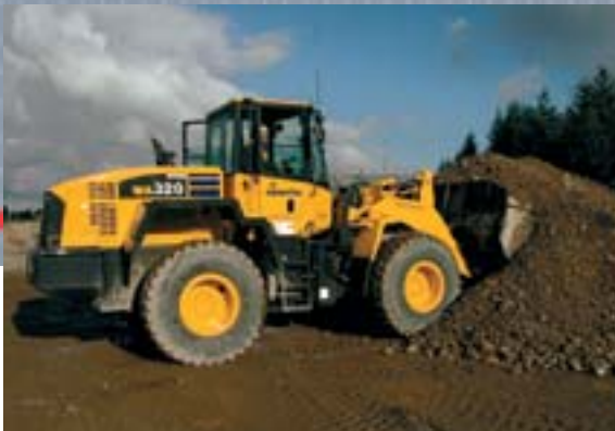
This Northwest Construction operator uses a Komatsu WA320-5 to move dirt at a retail development in Tacoma.
